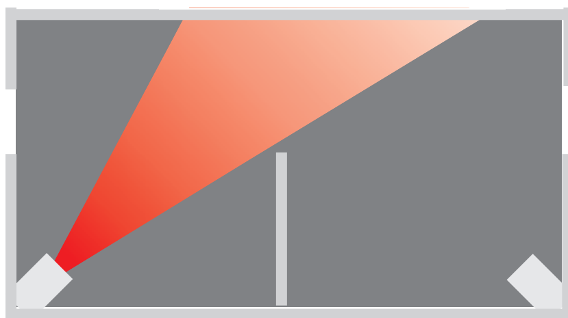
Without smoke: Chamber is designed so that light from the IR-LED does not reach the receiver
