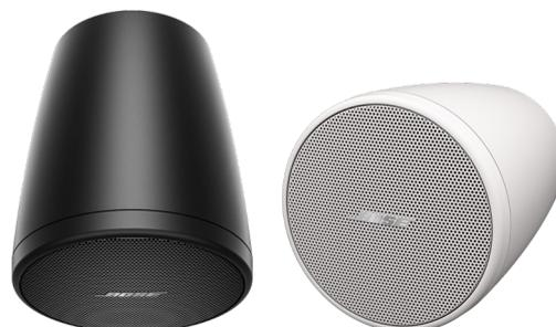
The FS2P is a dedicated pendant model with a full-range 2.25-inch transducer, low frequency range down to 83 Hz, and sensitivity of 87 dB SPL / 1W @ 1m.
